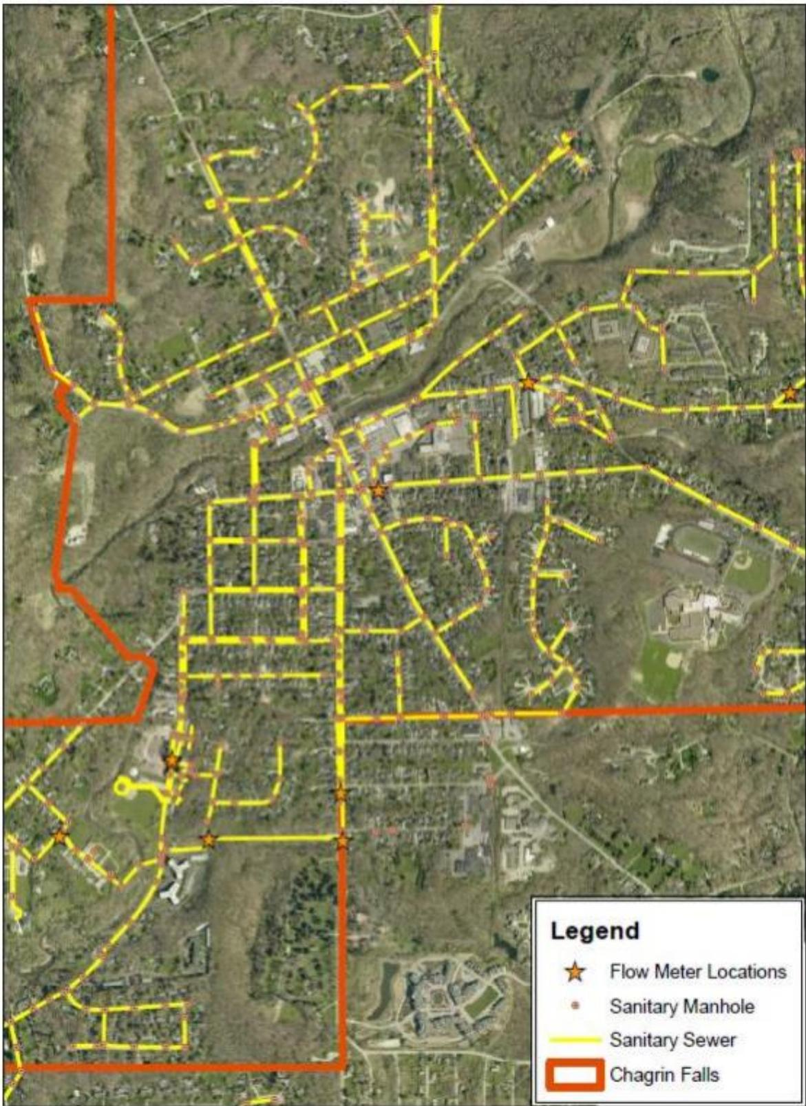
**Figure 3.** Map of Chagrin Falls showing sanitary sewer pipe alignments and flow meter locations
